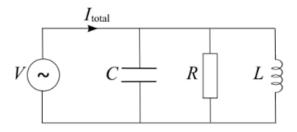
Consider the circuit in the diagram. A sinusoidal voltage of angular frequency  $\omega$ ,  $V = V_0 \cos(\omega t)$ , is applied to the circuit. Find a general expression for  $I_{\text{total}}$ , the current drawn from the voltage source. Sketch the amplitude and phase of the current as a function of the angular frequency.
